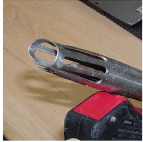
Photo 3 – Side view of retro-jet showing proximity of retro-jet nozzle to end of baffle. (approx 3 cm)
