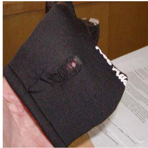
Photo 5 – Diver's glove showing hole at location of injection
