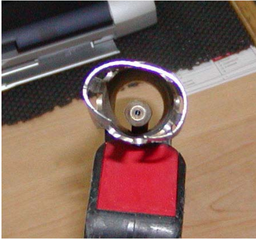
Photo 2 – End view of retro-jet
